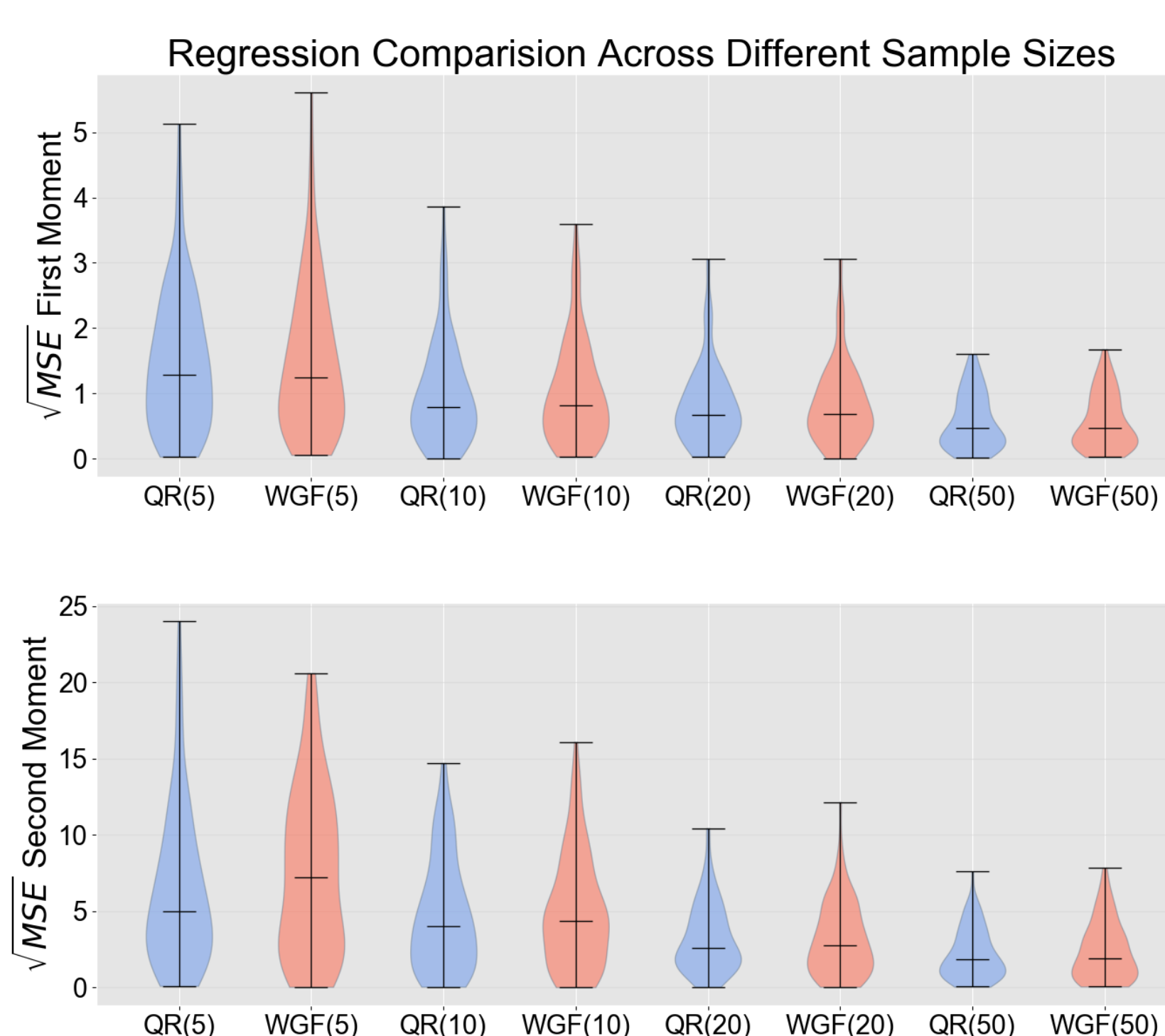
Figure 1: Error comparison of moment estimates: Violin plots of the estimation error in the first two moments using quantile regression and Wasserstein Gradient Flow regression are shown. The number of regressed samples is shown in parentheses.
